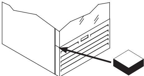
Insert between glass door and motor space the wood part to avoid door frame foldings during transport.
